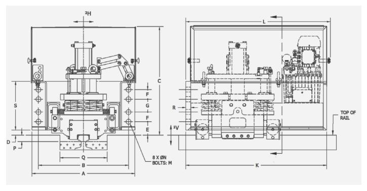
V Vertical Rail Deviation (Float) ±25mm relative to Rail Clamp enclosure at full rated capacity.
